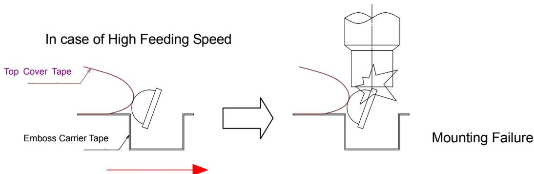
Even when the LED is in contact with the top cover tape; however, by lowering the feeding speed, it can be detached from the tape before absorbed by the nozzle.
