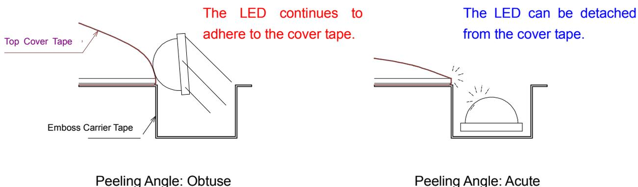
The peeling angle can be adjusted to its optimal value by some of the mounters as follows:
