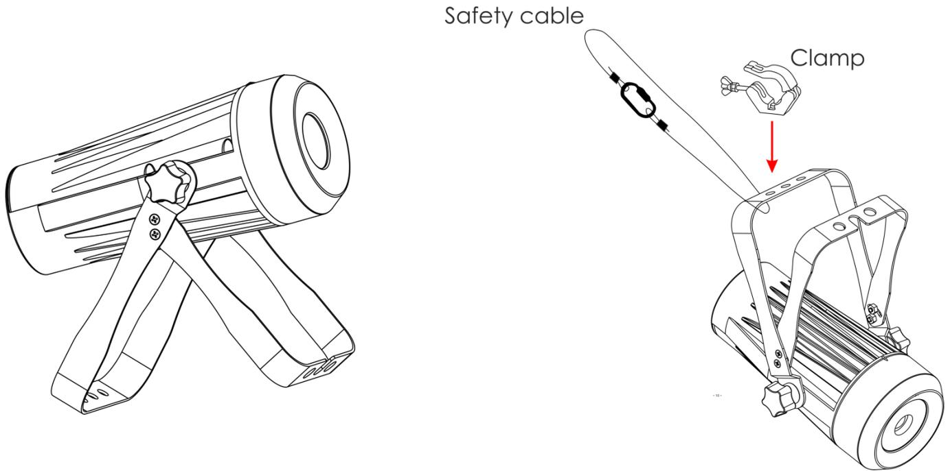
The Spectral M300 Q4 MKII can be placed on a flat stage floor or mounted to any kind of truss with a clamp.
