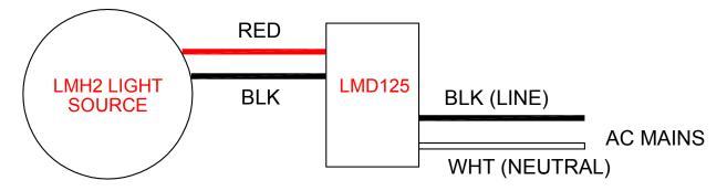
For the 230-V LMD125 and LMD300 LED power supplies, module operation is accomplished by connecting the AC mains to the appropriate terminal block pins.
