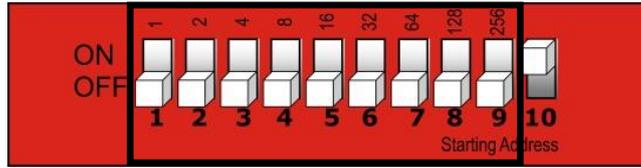
You need to know that DMX address settings are the sum of the dip switch values. A standard DMX address for a Showtec Swing 4, which has 6 channels is as follow:
